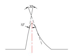
REMFORM® ||TM "F" The asymmetrical Unique Radius Flank™ thread form has the thread- forming advantages of a 30° thread, without the difficulty of manufacturing a 30° thread.
