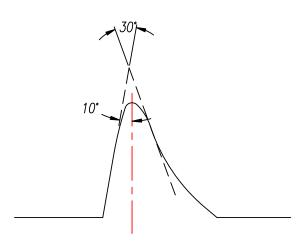
The REMFORM® II™ "HS" unique asymmetrical radius flank thread form has the thread forming advantages of a 30° thread, without the difficulty of manufacturing a 30° thread.
